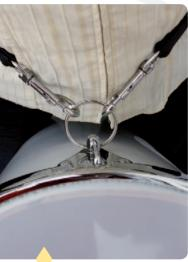
The instrument can be fastened by using either two karabiner snap-links or one ring affixed centrally. An exact description can be found in the adjusting-guidelines.
